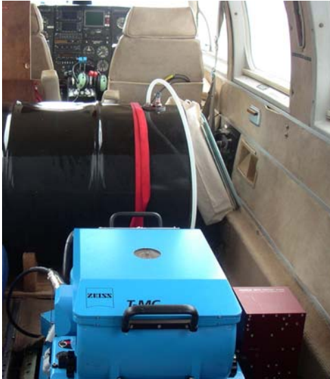
Figure 6: Interior of Scankorts Piper Navajo, equipped with a RMK-TOP 15 with IGI IMU-IIid
