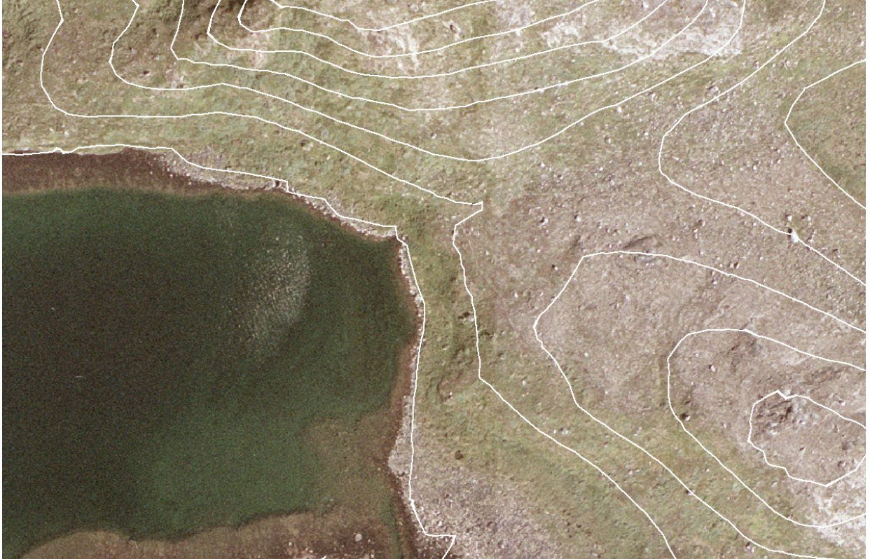
Figure 8: Mosaic of two orthophotos with superposed contour lines of the Qaqortoq area (Julianehaab). Height model and exterior orientation based on AEROcontrol data. Copyright Scankort A/S 2003.
