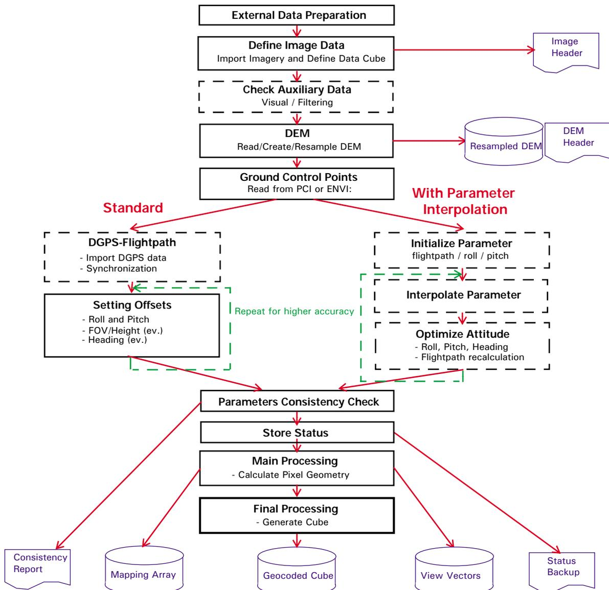
Figure 2: Process data flow of the parametric geocoding as implemented in the PARGE application, including the final outputs of the process.
