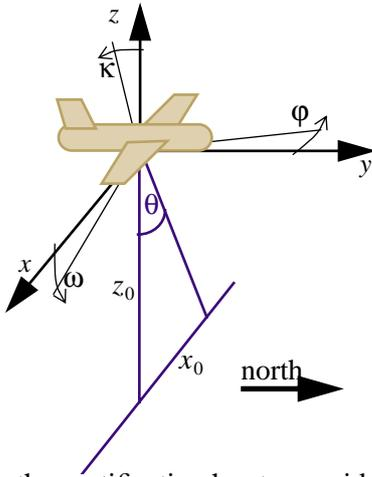
Figure 1: Chosen north facing coordinate system for the PARGE application and theoretical scan situation (situation before virtually turning the aircraft).
