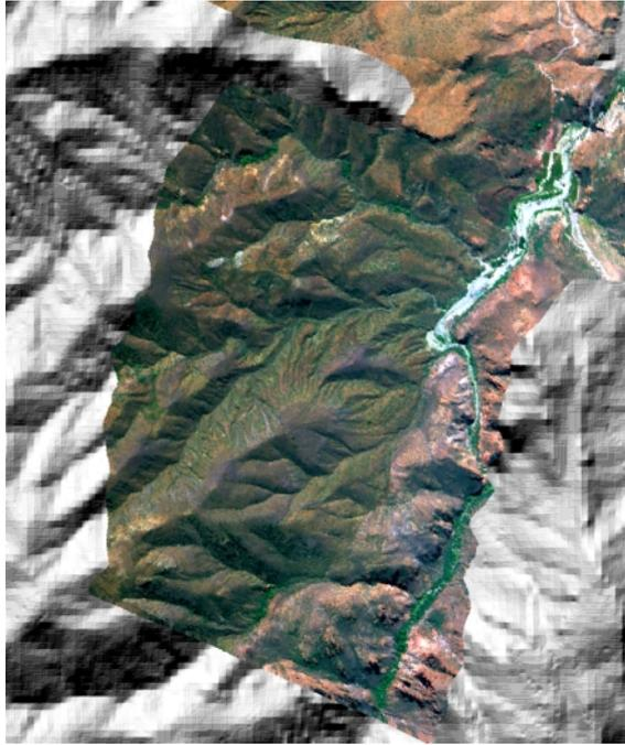
Figure 3: Overlay of the ortho-rectified AVIRIS low altitude imagery on the illumination-shaded USGS DEM.
